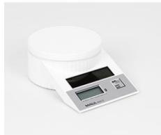
For demonstration and student experiments, with 4-digit LCD display (easy, mirror-free reading through sharply slanted display), automatic switch-off, automatic reset and hold key to freeze the displayed weight. Powered by solar cells, excess energy is stored and used in low light conditions (below 150 lux). Stable housing made of unbreakable plastic. Made in Germany with patented measuring system.
