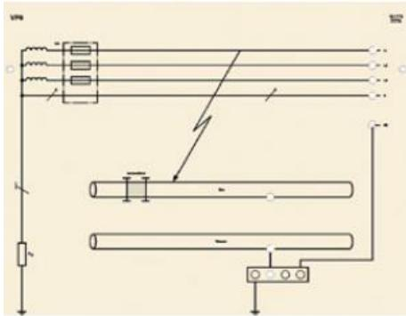
P 9 Mask: TT-System net with earth fault in consumer devices with and without potential equalization
