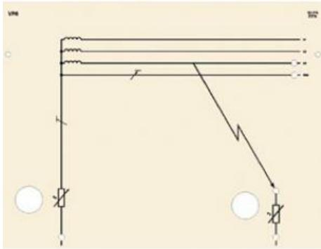
VP 6 Mask: Voltage limitation in the event of a grounding fault of an outer conductor
