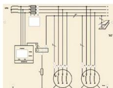
VP 5 Mask: The IT-System with isolation monitoring device and additional potential compensation
