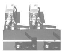
Figure 1-8: Parts manipulators (flippers)
