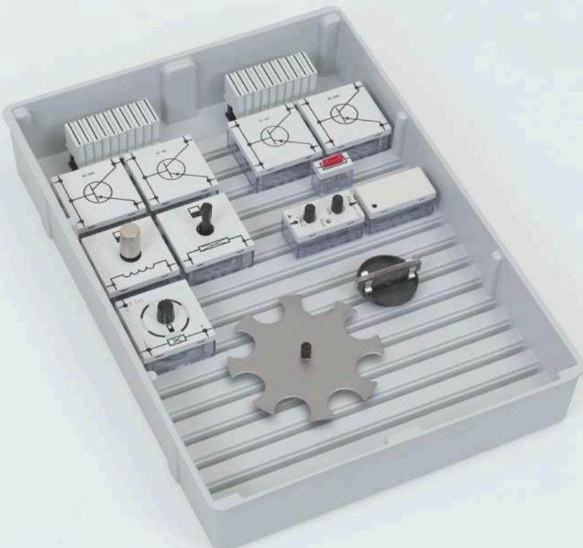
The STE elements come ready for operation and assembly with their electrical and electronic components encased in transparent housings to protect against external mechanical damage. Thanks to the transparent bottom part the original component is visible.
