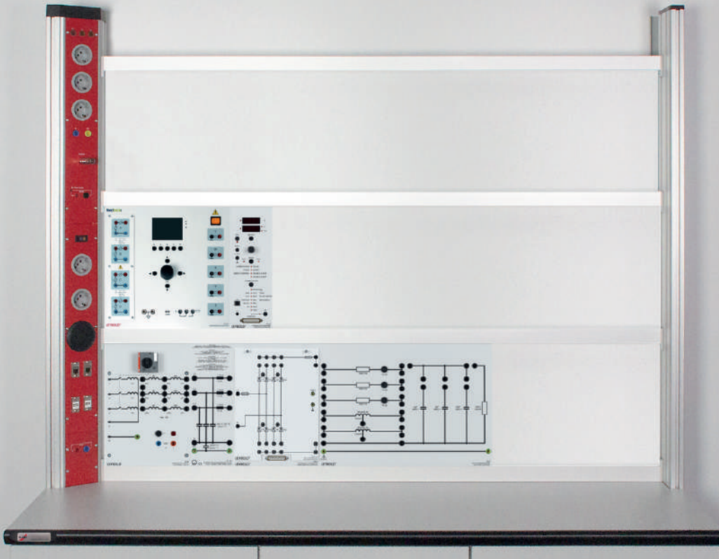
Static / Controlled converter valves (E2.4.2.1)
