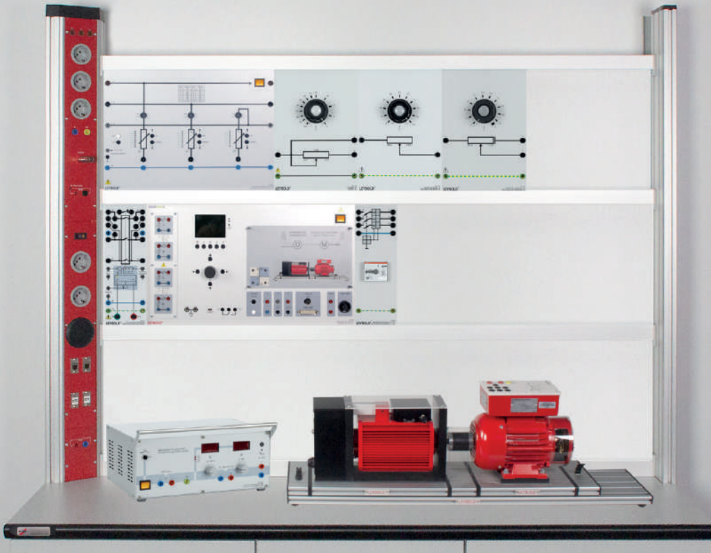
DC compound machine, 0.3 (E2.2.2.1)
